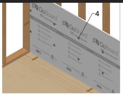
4. Install remaining washers spaced 12" apart in the interior area (field) of board. To ensure a waterproof installation, GoBoard Washers should only be installed around board perimeters AFTER GoBoard Sealant has been applied.
